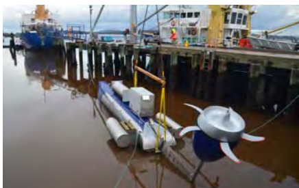
MAKO turbine and test rig being launched for endurance testing
